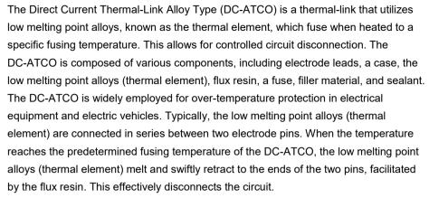
The SETsafe | SETfuse Direct Current Thermal-Link (Alloy Type) is available in axial and radial shapes, with a Rated Functioning Temperature ranging from 102 °C to 187 °C, Rated Current 15 A, Rated Voltage 850 VDC. It is compliant with RoHS and REACH regulations.
